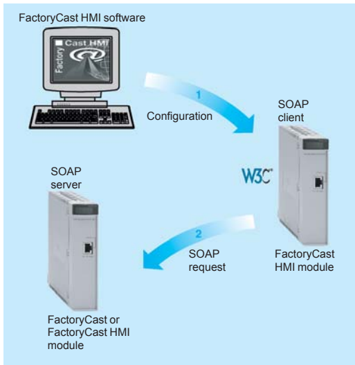
ModbusXMLDa client interface
